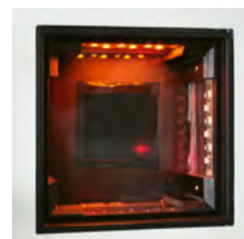
The daphnia behaviour in sample water is observed in the measuring chamber by a CCD camera.
