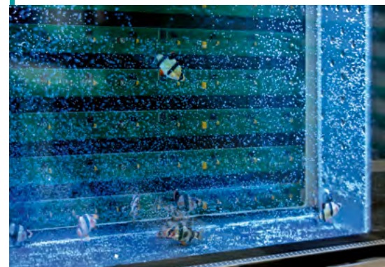
The ToxProtect II monitors the swimming activity of fish in an aquarium fed with drinking or mains water.
