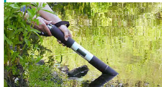
AlgaeTorch measurement on site.
