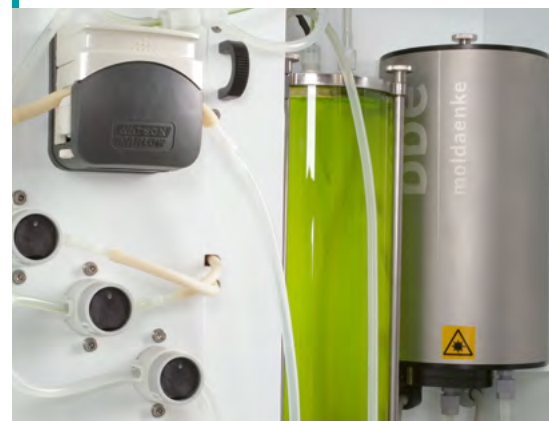
Sample water is mixed with the algae test solution and then analysed.
