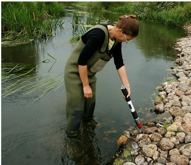
BenthoTorch used in the AQUAREHAB project in Denmark and Belgium
