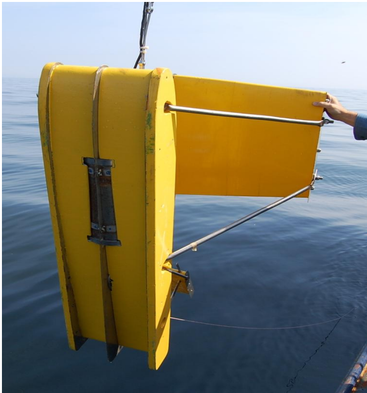
Towed undulating system measuring T, S, Chl a and phycosyanin
