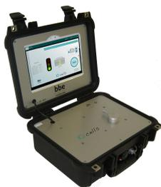
bbe 10cells for ballast water testing
