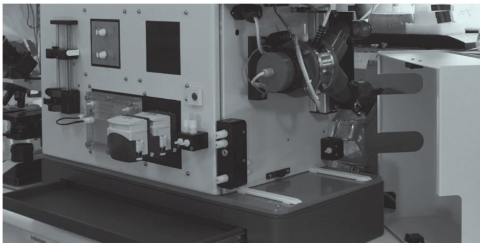
Daphnia Toximeter II with drip pan, pumpheads and filter unit
